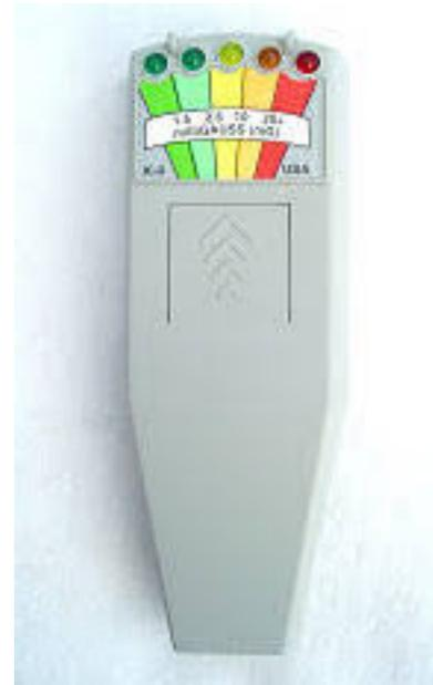
fields. The electric field is constant, static and is based on the total amount of electrical charge present. The magnetic field fluctuates and is based on the actual flow of electricity. The K-II meter can only measure magnetic fields. Other more expensive meters can measure static electric fields or both.
